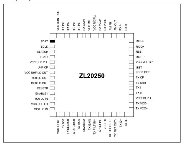
Figure 2 - ZL20250 Package Diagram
