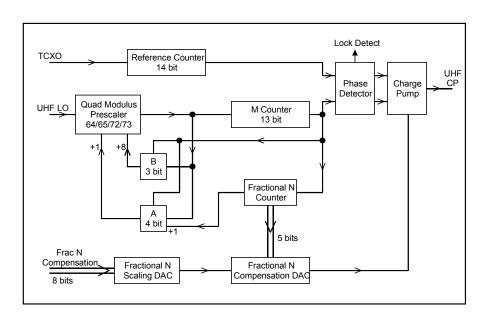
Figure 9 - UHF Synthesizer
