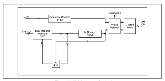
Figure 12 - VHF Frequency Synthesizer
