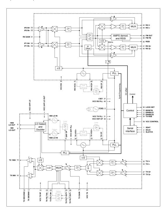
Figure 3 - ZL20250 Detailed Block Diagram
