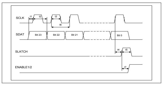
Figure 13 - Serial Bus Timing
