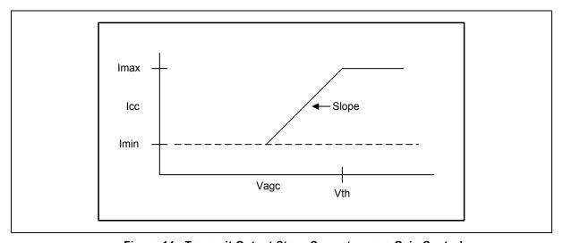
Figure 14 - Transmit Output Stage Current versus Gain Control
