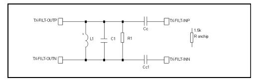
Figure 8 - External Transmit IF Filter
